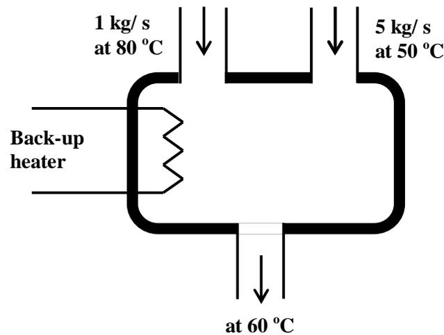
There is no accumulation of water in the tank. A back-up heater is provided to ensure a constant outflow temperature of water at 60 °C from the tank under steady state. What is the required capacity of the back-up heater to the nearest kW? \_\_\_\_\_
