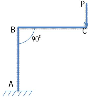
Q.17 Neglecting the axial compression of member AB, the deflection of point C in the direction of the load is
