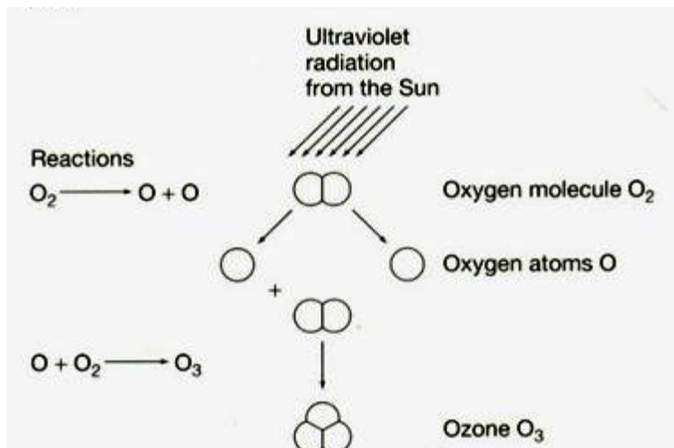
Figure showing the production of ozone in the upper atmosphere from photolysis caused by ultraviolet radiation from the Sun.
